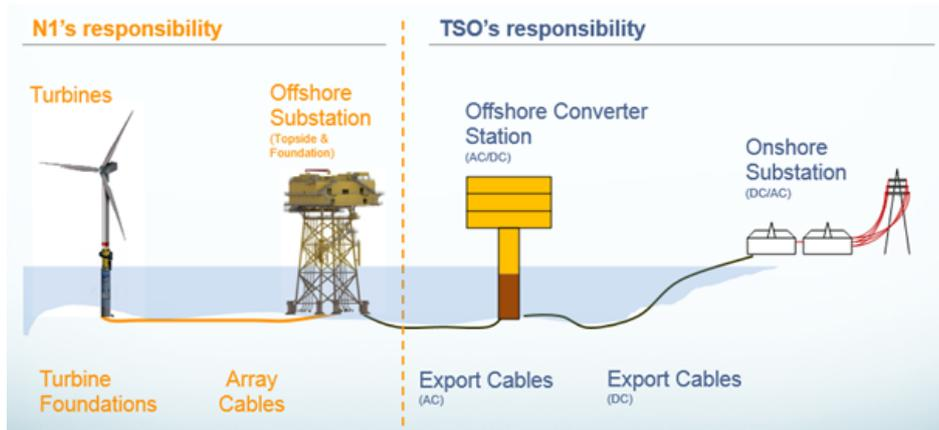
Figure 23: Overview of the different cable distributor stations on- and off-shore. The Offshore Substation is relevant for the optimization of the cable lengths in this thesis, as it connects the cable network to the individual turbines. Source: [1].
