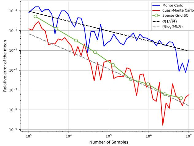
Figure 9.: Convergence behavior of the presented methods in terms of the relative error in the mean w.r.t to the quasi-Monte Carlo reference solution.
