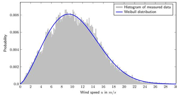
Figure 3.: Wind speed measurements at the FINO3 research platform at a height of 100 m for the eight years from January 2010 to December 2017 for the western wind direction sector ( $255^\circ$  to  $285^\circ$ ). The data is fitted by a Weibull distribution using the maximum likelihood estimation.
