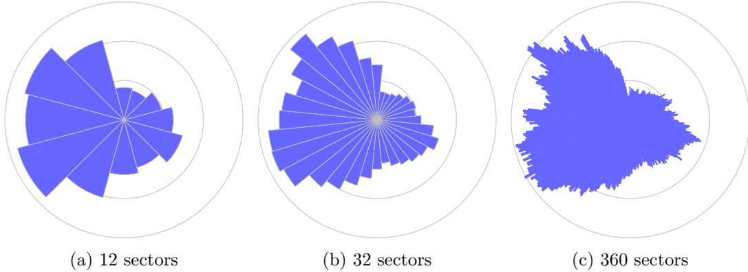
Figure 2.: Wind direction measurements at the FINO3 research platform in the North Sea, about 80 km away from the German island Sylt. The measurements at a 100 m height taken over eight years from January 2010 to December 2017 are clustered into  $N_{\text{dir}}=12$ , 32, and 360 direction sectors.
