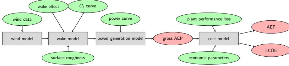
Figure 1.: Structure of the offshore wind farm model. Input parameters are highlighted in green. These parameters are also later used for the uncertainty quantification. Possible outputs of the wind farm model (highlighted in red) are the annual energy production (AEP) and the levelized cost of electricity (LCOE).
