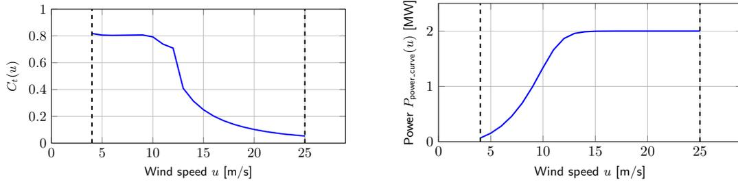
Figure 5.: Thrust coefficient  $C_t$  and power production of the turbine Vestas V80 with cut-in speed of 4 m/s and cut-out speed of 25 m/s (dashed vertical lines).
