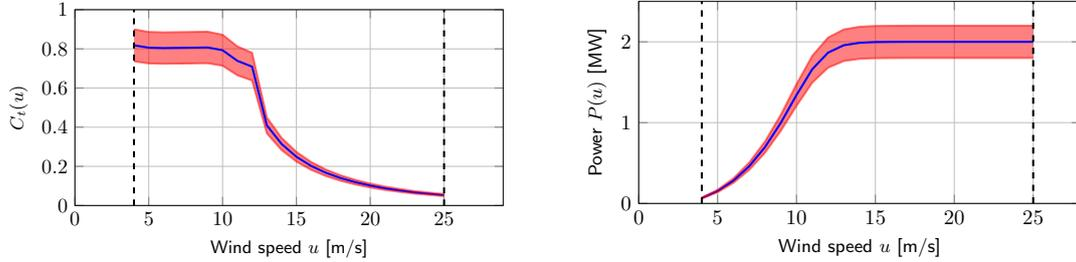
Figure 7.: Exemplary disturbed  $C_t$  and power curve of a Vestas V80 turbine with a cut-in speed of 4 m/s and cut-out speed of 25 m/s (dashed vertical lines). The red tube illustrates the  $C_t$  and power curve with a disturbance of  $\pm 10\%$ .
