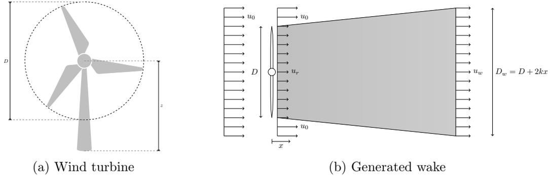
Figure 4.: Wind turbine with hub height  $z$  and rotor diameter  $D$ . The wake diameter  $D_w$  grows linearly by  $2k$ . Inside the wake, the incident wind speed  $u_0$  is reduced to the wake velocity  $u_w$ . The Figures are taken from Heiming (2015).
