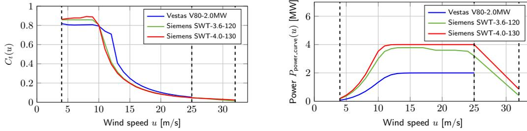
Figure 12.: Thrust coefficient  $C_t$  (left) and power production (right) of the turbines Vestas V80 by L. Jensen et al. (2004), Siemens SWT-3.6-120, and Siemens SWT-4.0-130. The dashed vertical lines show the cut-in and cut-out speeds.
