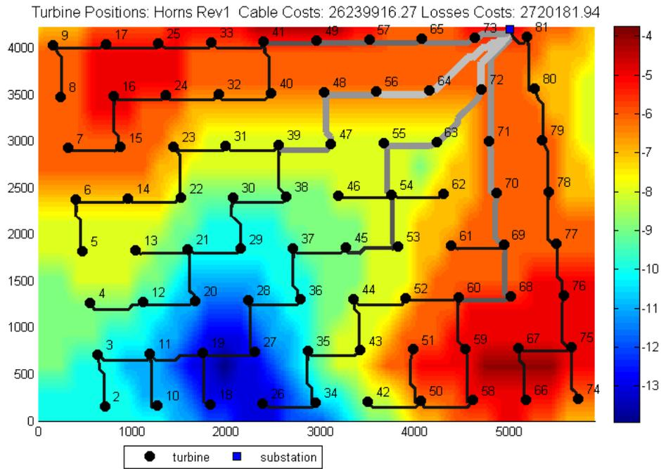
Figure 17: Optimized layout of Horns Rev not considering connection costs, costs in €
