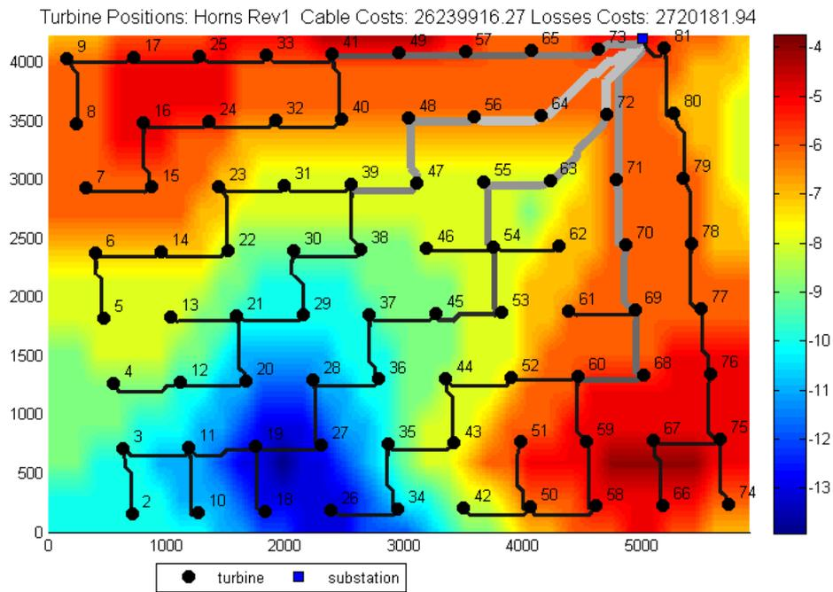
Figure 16: Optimized layout of Horns Rev considering power losses, costs in €
