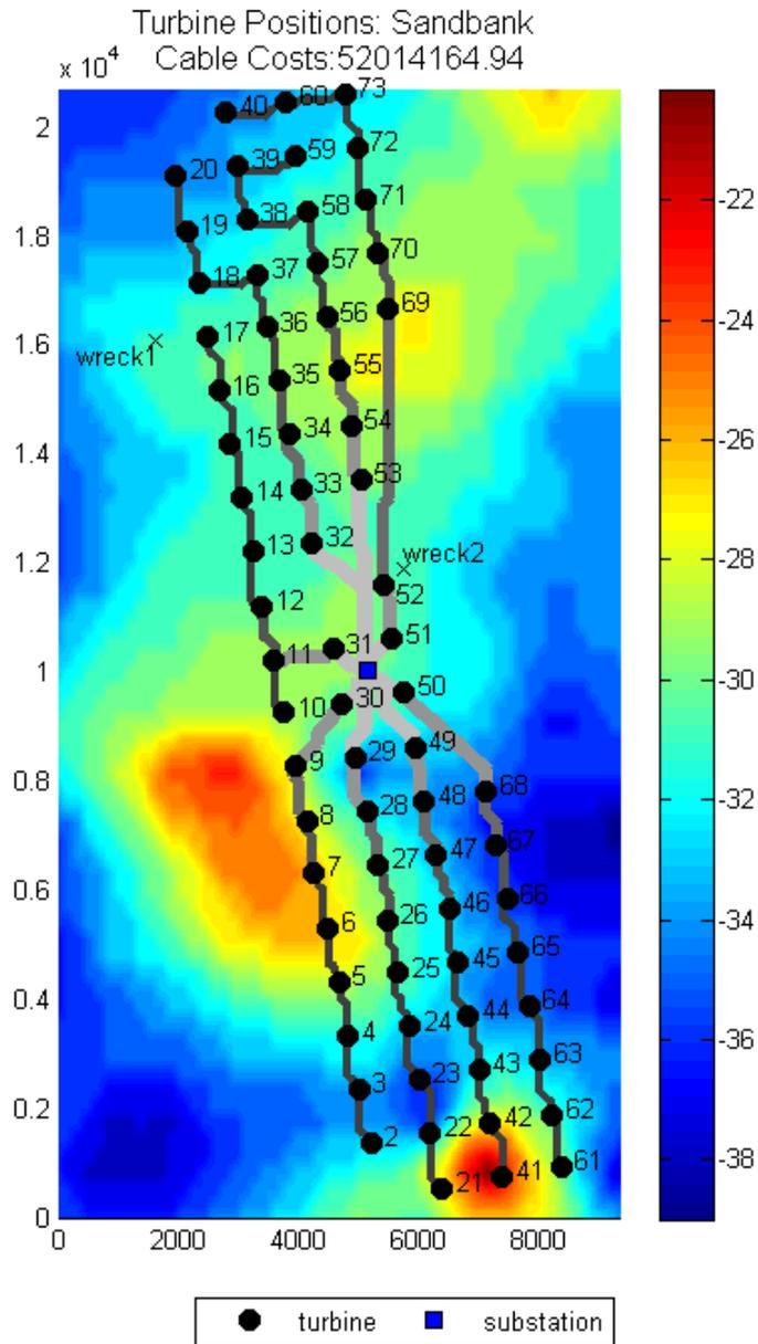
Figure 12: Optimal layout of Sandbank considering the constraints from Step 1, cable costs in €
