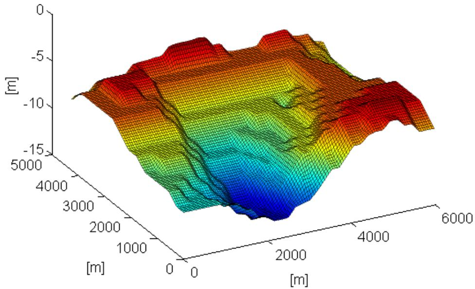
Figure 6: Topography of the Horns Rev wind farm
