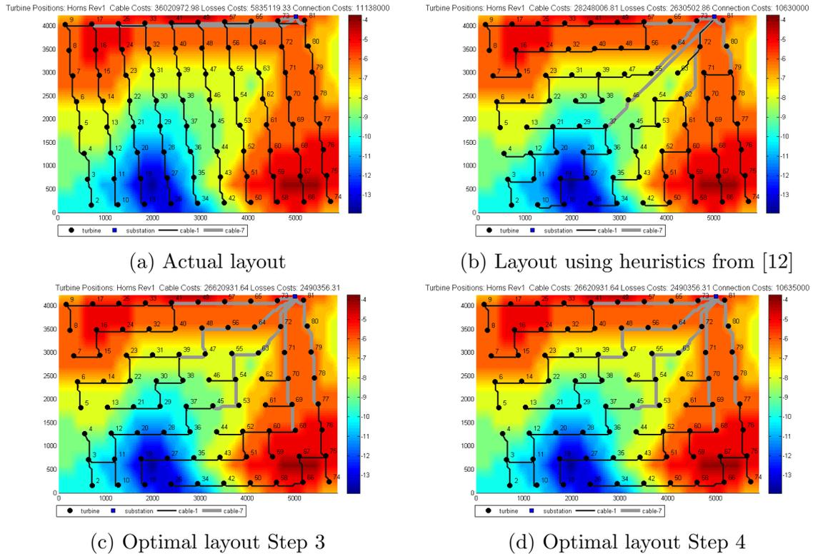
Figure 19: Comparison of Horns Rev cabling layouts, costs in €
