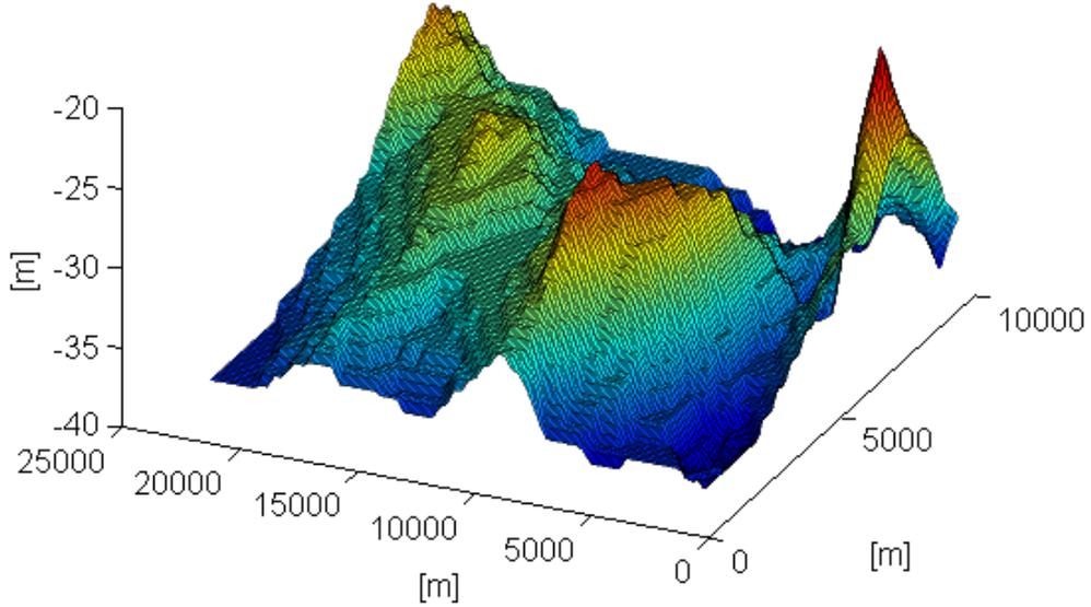
Figure 7: Topography of the Sandbank wind farm
