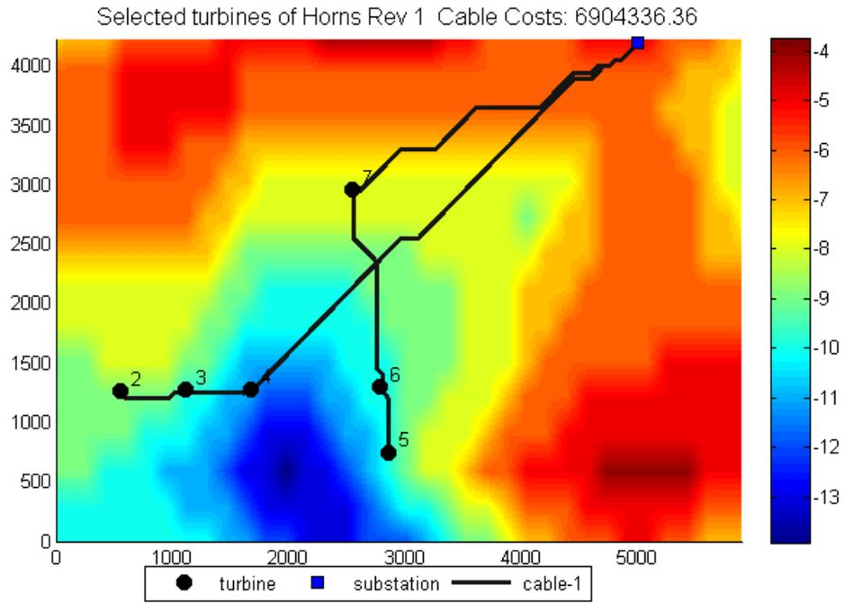
Figure 13: Optimal layout with crossings, cable costs in €
