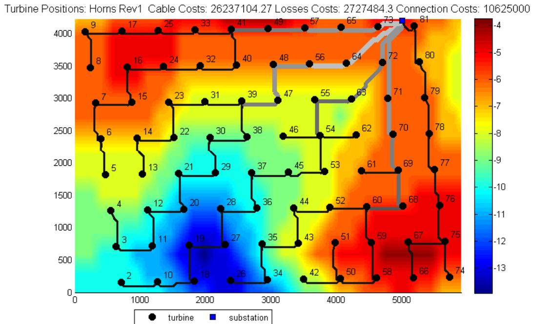
Figure 18: Optimized layout of Horns Rev considering connection costs, costs in €
