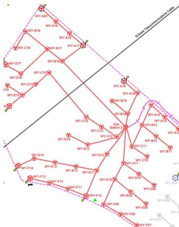
Figure 10: Grid of the offshore wind farm Walney 2, cf. [21]
