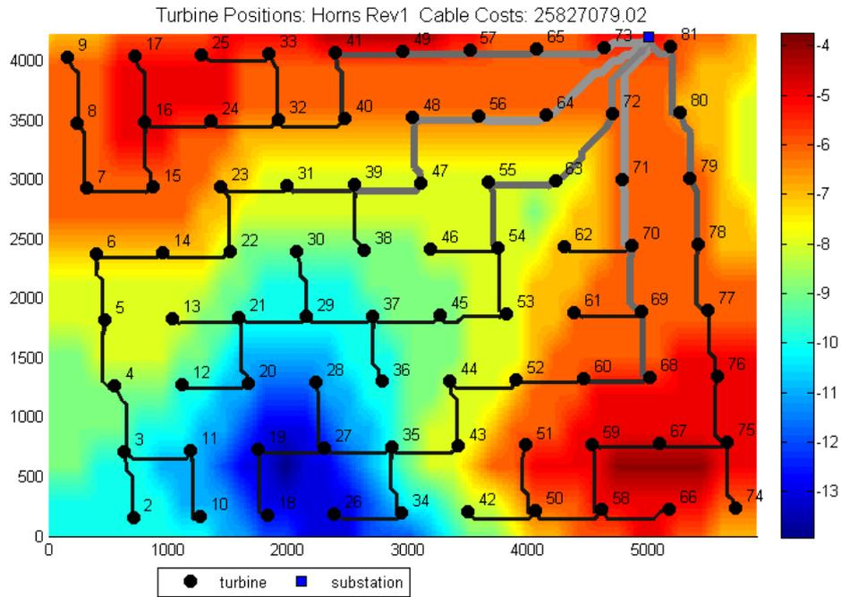
Figure 11: Optimal layout of Horns Rev wind farm considering the constraints from Step 1, cable costs in €
