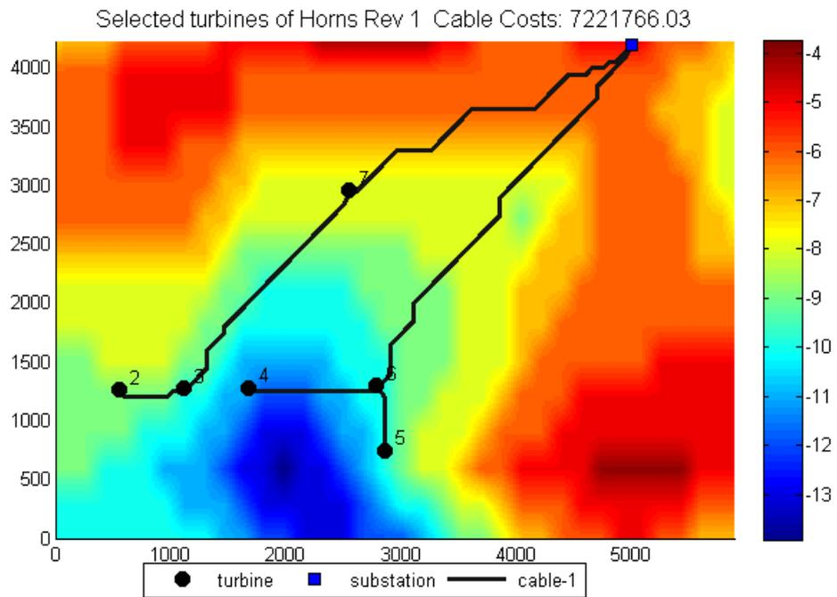
Figure 14: Optimal layout without crossings, cable costs in €
