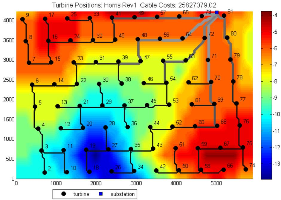
Figure 15: Optimized layout of Horns Rev not considering power losses, costs in €
