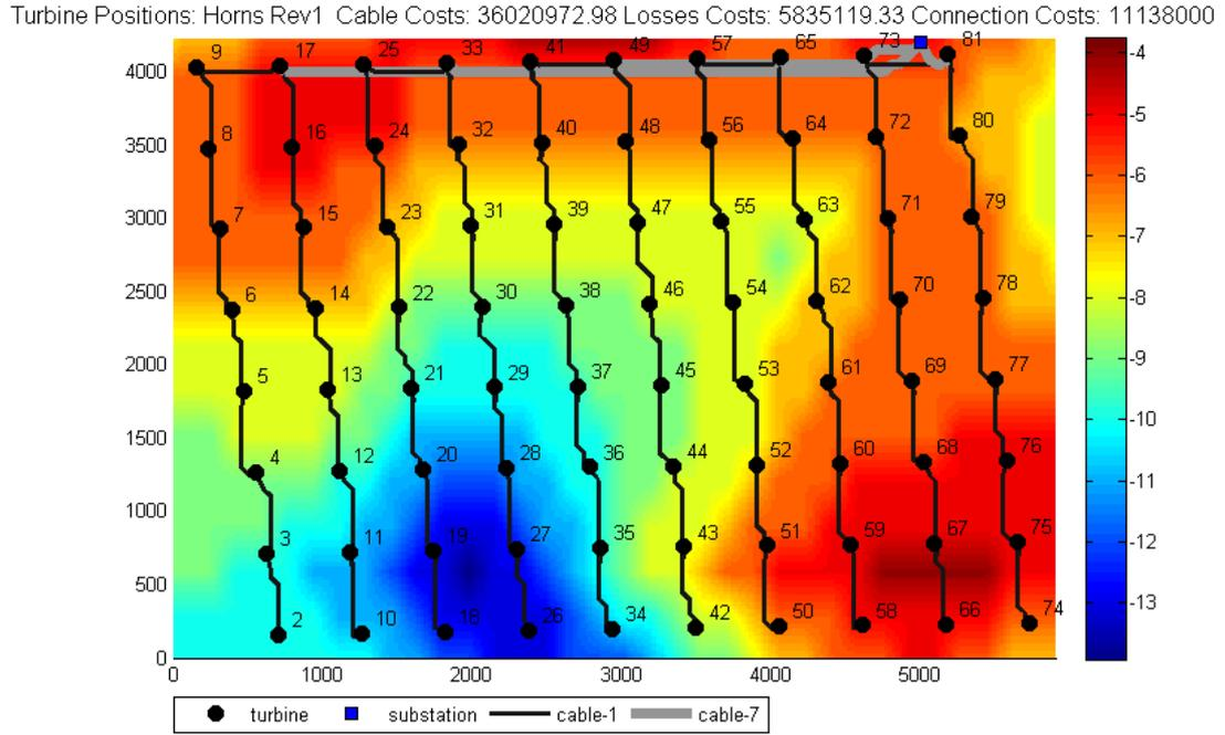
Figure 8: Actual layout of Horns Rev wind farm cf. [7], costs in €
