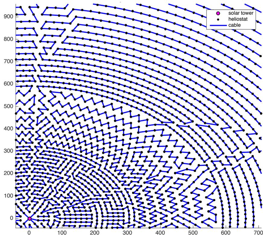
Figure 38: Solar tower: DLR Field, country: Spain. A segment of the optimized layout with the help of the shortest distance algorithm and the 2-opt heuristic.
