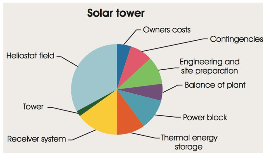
Figure 2: Total costs of a solar tower power plant in South Africa, cf. [17]. The heliostat field including cabling aggregates approximately one third of the total costs.
