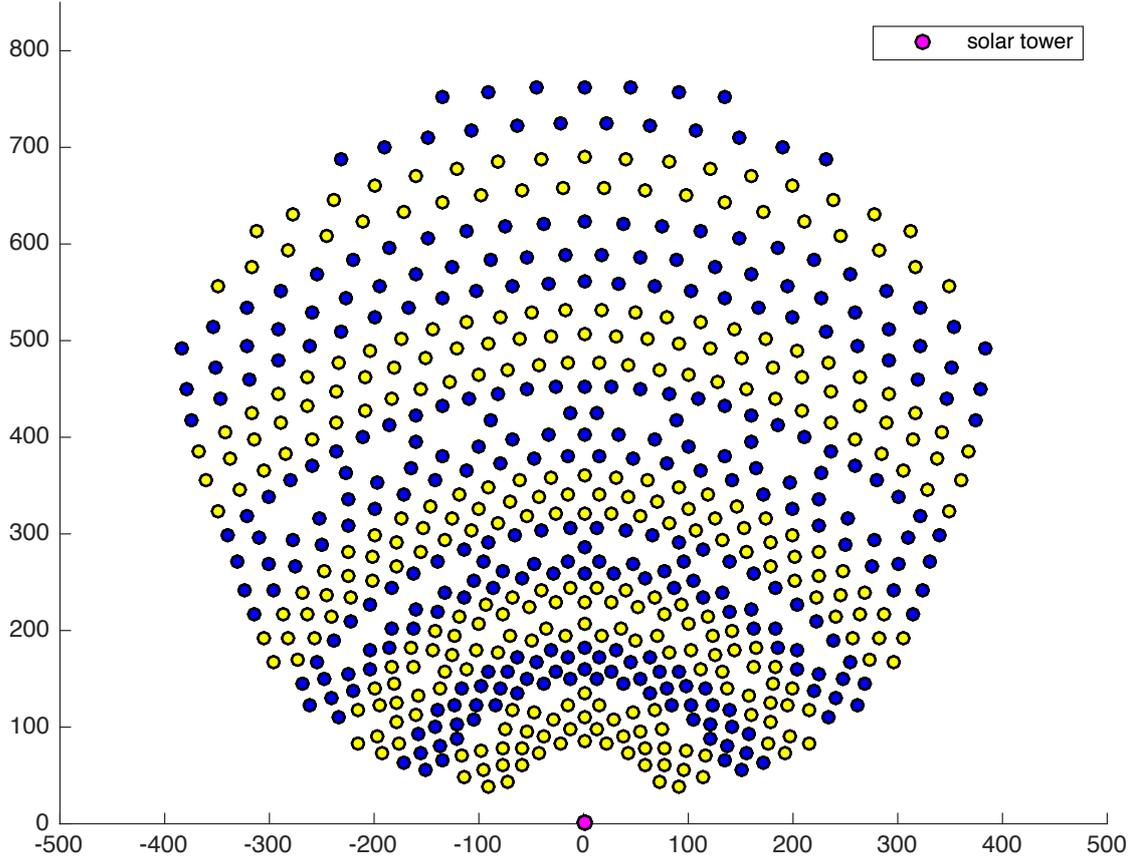
Figure 16: Solar tower: PS10. In a first step the algorithm creates belts. The corresponding heliostats are visualized in yellow and blue.
