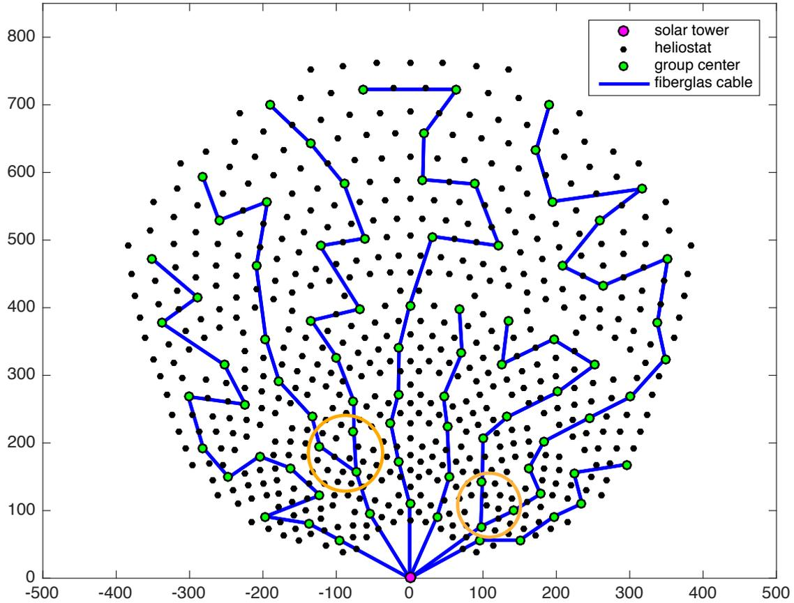
Figure 21: Solar tower: PS10, country: Spain, fiberglass cable length: 6 395.1m, trench length: 6 097.39m, costs for fiberglass cable and switches: 219 419.73€. Applying Esau Williams Version 2 on the computed centers of the groups. New cable connections can be seen in the orange circles. Some cables are installed parallel to avoid crossings of copper and fiberglass cables. Thus trench and cable length differ.
