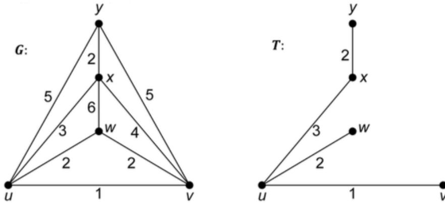
Figure 11: An exemplary graph  $G$  and its minimum spanning tree  $T$  computed with Kruskal's algorithm, cf. [9].
