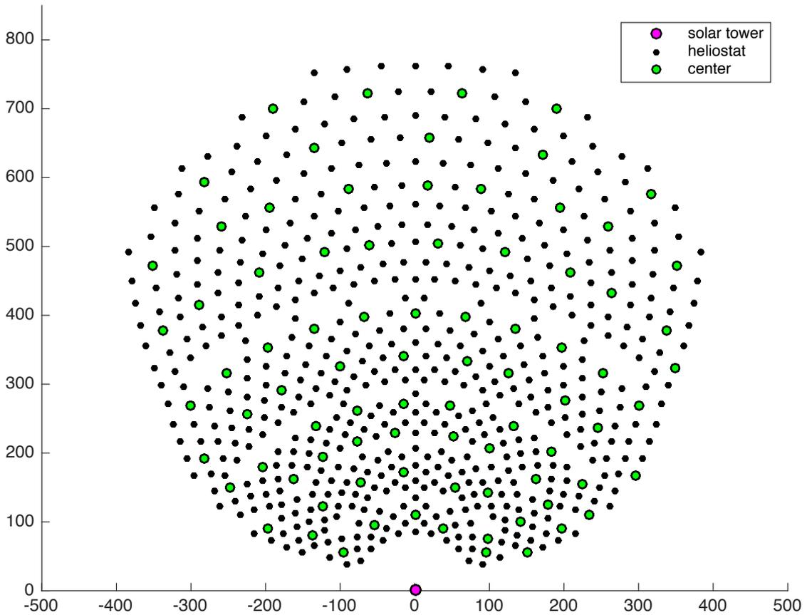
Figure 18: Solar tower: PS10. The centers of the groups of  $b_{\max\text{CU}} = 8$  are highlighted in green.
