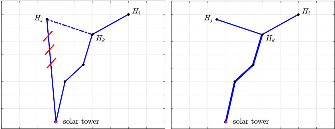
(a) Crossings may occur if heliostat  $H_j$  does not lay in the most inner circle and has the solar tower as predecessor. Instead it shall be connected to the nearest heliostat. (b) Revised version. Heliostat  $H_j$  is connected to  $H_k$  instead of the solar tower. The thicker lines represent two cables being laid parallel.
