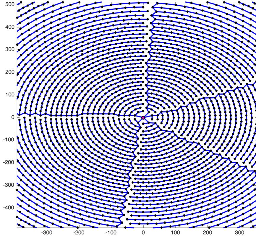
Figure 37: Solar tower: DLR Field, country: Spain. A segment of the naive layout of the data cable for the DLR Field.
