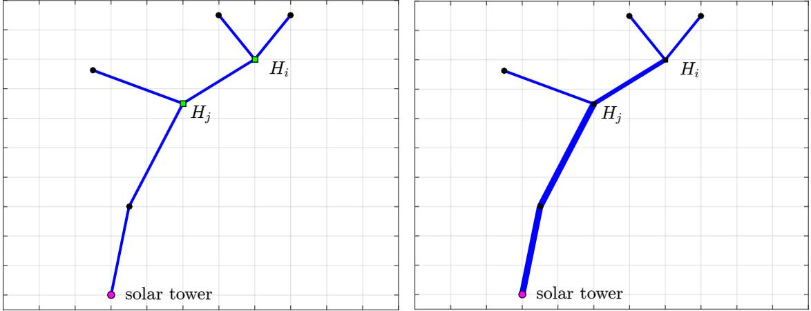
(a) Option 1: A switch of type *branching fiber-glas* is installed at heliostats  $H_i$  and  $H_j$  (green square).
