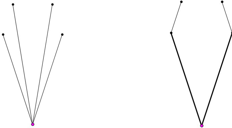
(a) At first each node is directly connected to the root node. (b) Result after applying the Esau Williams heuristic.
