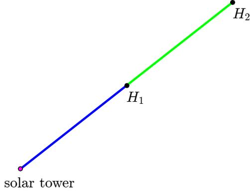
Figure 29: The blue cable powers  $H_1$  and  $H_2$  (200 W in total) while the green one powers  $H_2$  only (100 W).
