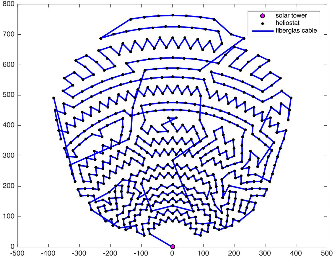
Figure 6: Solar tower: PS10, country: Spain, fiberglass cable length: 18 421.19m, total costs: 596 614.63€. Hamiltonian path computed with the nearest neighbor algorithm. Several crossings as well as long connections occur.
