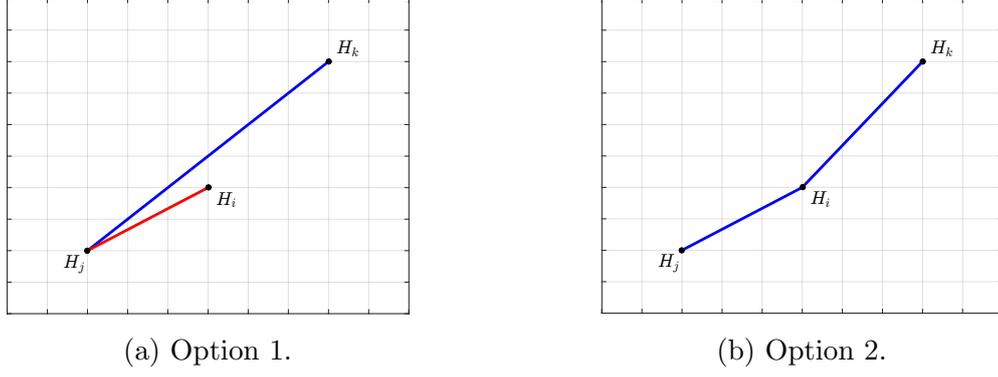
Figure 23: Example for cabling that could be replaced by a shorter and more economic alternative. One square in the grid has a side length of 20 meters.
