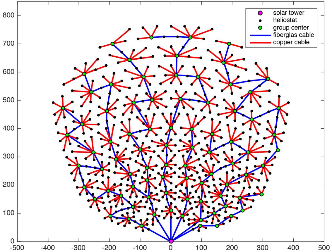
Figure 24: Solar tower: PS10, country: Spain, fiberglass cable length: 6 402.2m, copper cable length: 16 640.8m, trench length: 22 745.29m, total costs: 690 912.38€. Final layout of step 5b. Each group member is connected to the center of its group with a copper cable and not sensible connections are removed.
