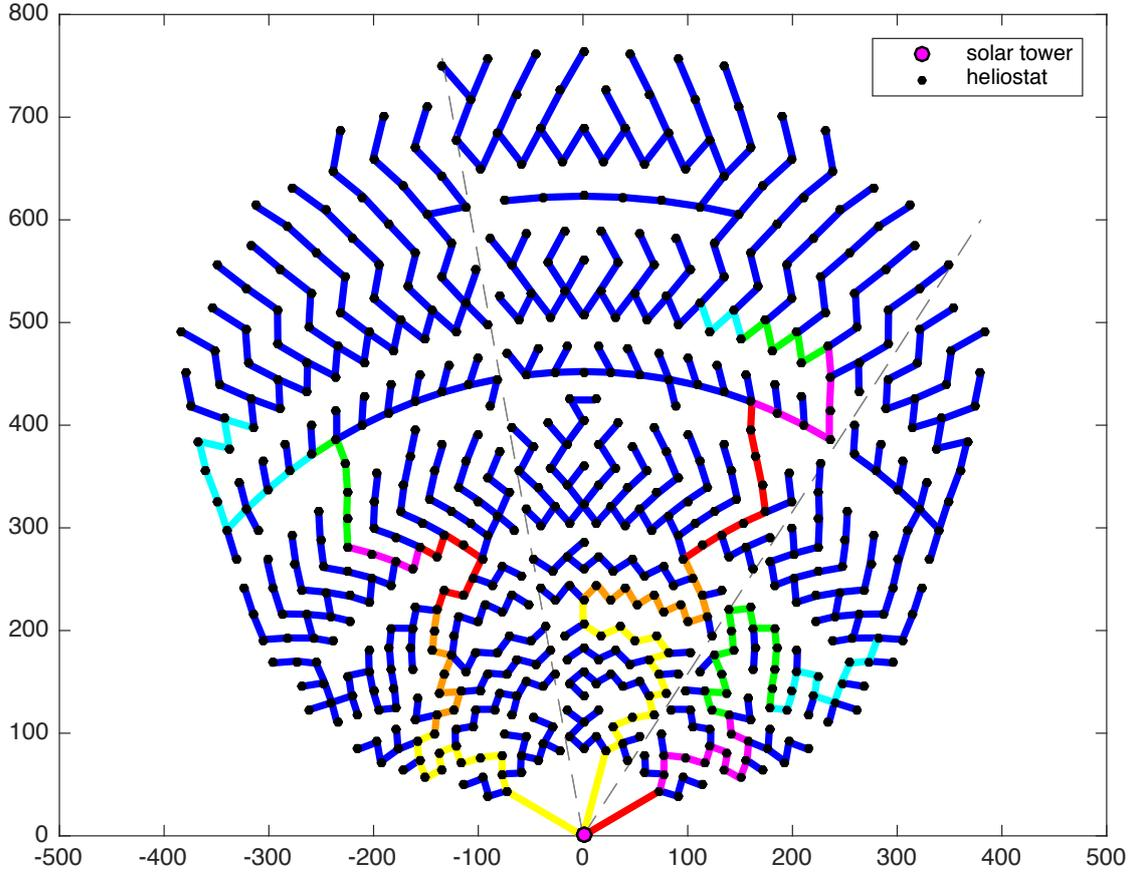
Figure 31: Solar tower: PS10, country: Spain, cable length: 16 214.4m, total costs: 455 647.73€. Three minimum spanning trees connecting each subsection with the solar tower. The cake pieces are indicated by grey dashed lines. Different colors of the cables mark different cable types.
