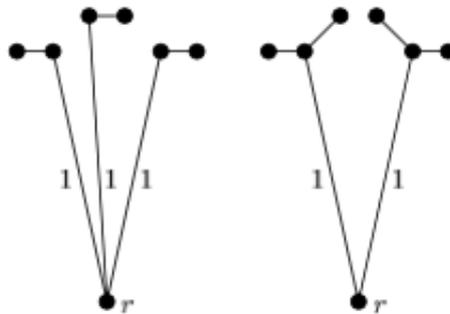
Figure 36: The left-hand side shows the result of applying Esau Williams heuristic to an exemplary graph while the right-hand side shows the optimal solution. Cable capacities  $k \in \{1, 2, 3\}$ ,  $k_{\max} = 3$ , are being used. Instead of the optimal solution containing two subtrees the solution generated with the help of Esau Williams algorithm creates three.
