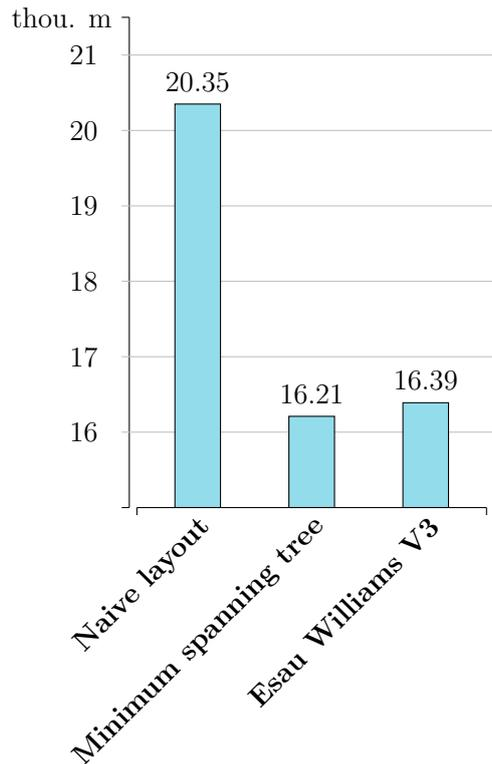
Figure 34: Solar tower: PS10, country: Spain. Comparison of the total cable length of the different results for the power cable in thousand meters.
