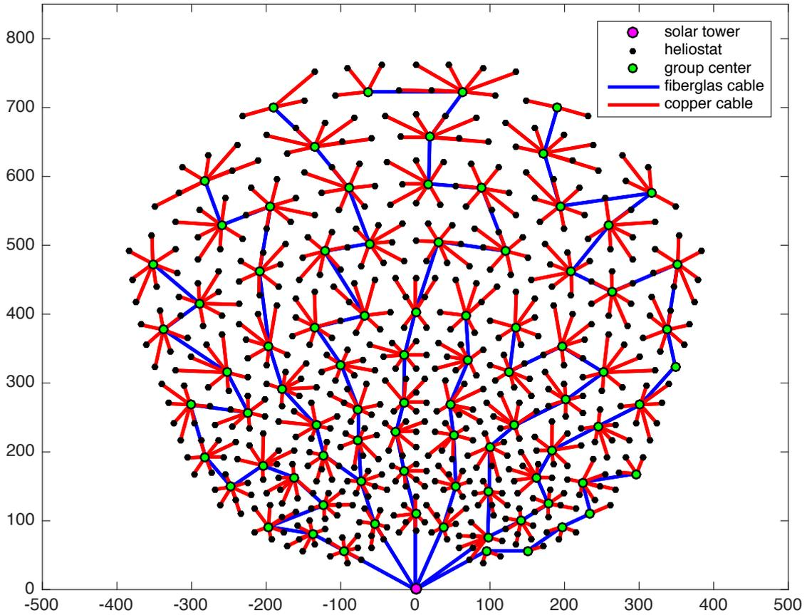
Figure 22: Solar tower: PS10, country: Spain, fiberglass cable length: 6 395.1m, copper cable length: 18 371.98m, trench length: 24 469.37m, total costs: 733 723.58€. Each center is connected with the other group members by a copper cable.
