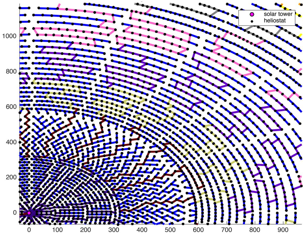
Figure 40: Solar tower: DLR Field, country: Spain. A segment of the layout of the power cable for the DLR Field generated by Kruskal's algorithm presented in Subsection 6.2. Different colors mark different cable types.
