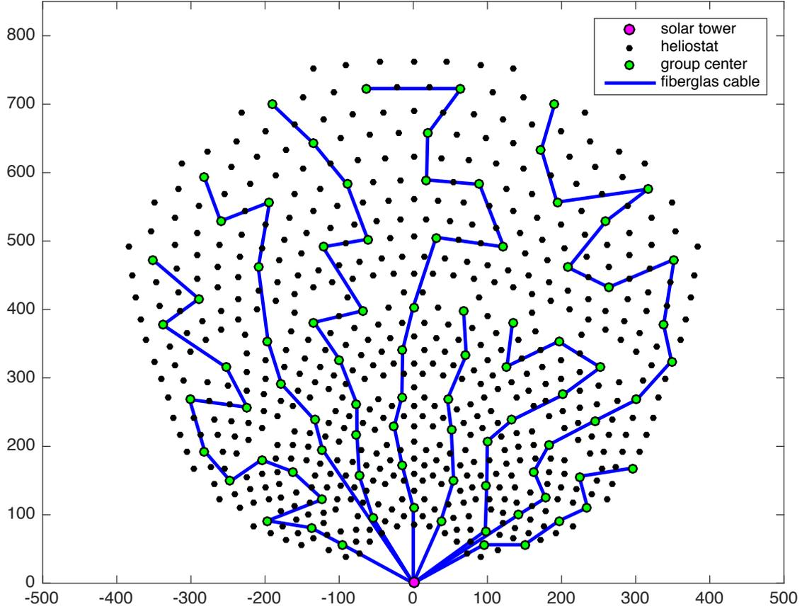
Figure 19: Solar tower: PS10, country: Spain, fiberglass cable length: 6 388.21m, costs for fiberglass cables and switches: 227 258.09€. Applying Esau Williams Version 2 to the centers of the groups. Two connections from belt two and belt three may still cause crossings.
