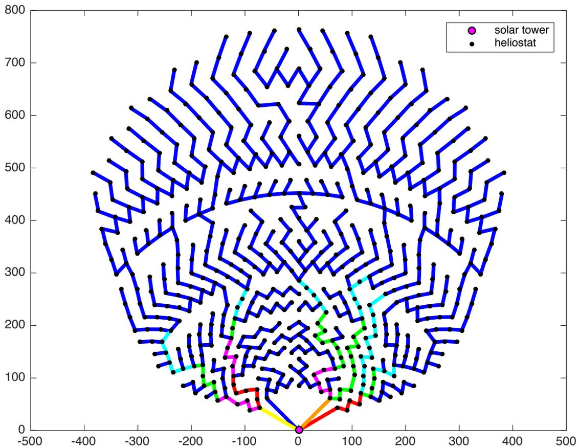
Figure 32: Solar tower: PS10, country: Spain, cable length: 16 388.92m, total costs: 454 665.39€. Result of applying Esau Williams Version 3 to the power cable.
