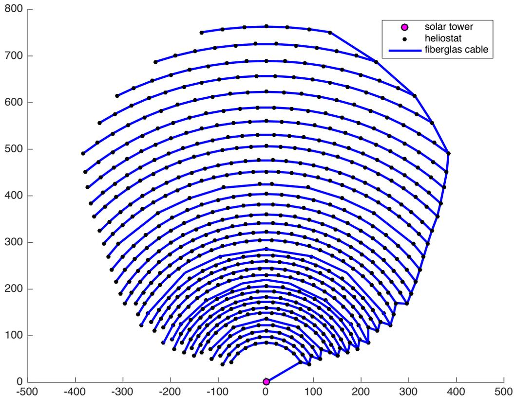
Figure 10: Solar tower: PS10, country: Spain, fiberglass cable length: 23 671.66m, trench length: 21 038.34m, total costs: 689 378.44€. Naive data cable layout of PS10 with the cables being installed in semi-circles.
