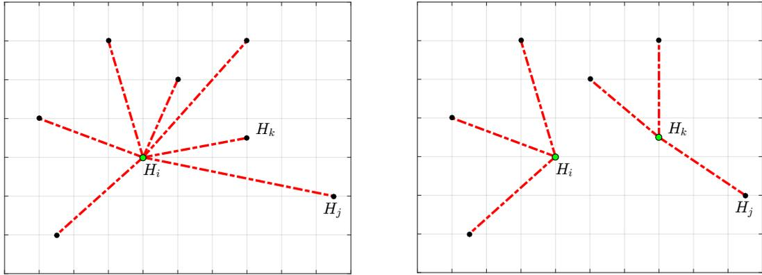
(a) The distance from heliostat  $H_i$  to heliostat  $H_j$  exceeds  $\ell_{\max} = 100$  meters. (b) Revised and permissible layout. No connection is longer than  $\ell_{\max} = 100$  meters.
