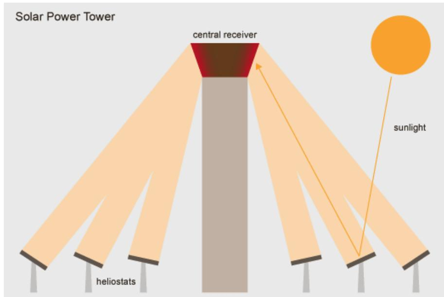
Figure 1: Layout of solar tower power plants, cf. [22]. The solar radiation is reflected by heliostats to a central receiver that is located at the top of the solar tower.
