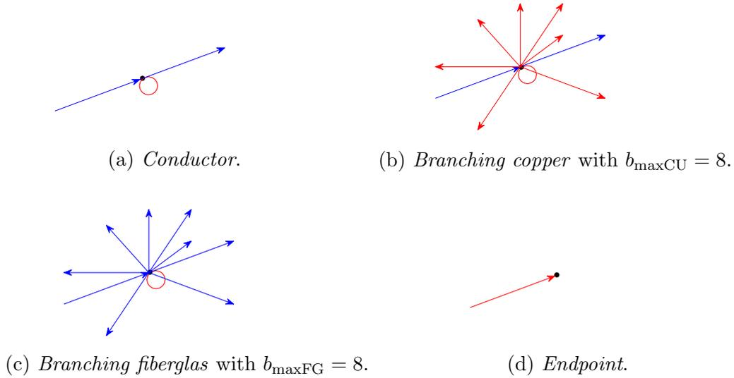
Figure 5: The LOCs that are used for the data cable. Fibreglas cable is represented by blue and copper cable by red arrows.
