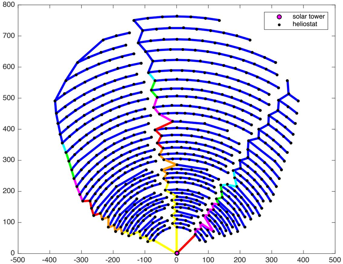
Figure 30: Solar tower: PS10, country: Spain, cable length: 20351.87m, total costs: 567979.63€. Naive power cable layout of PS10.
