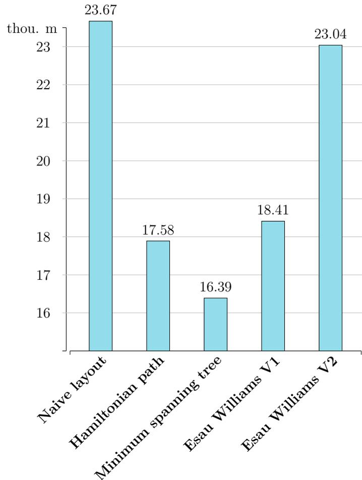
Figure 27: Solar tower: PS10, country: Spain. Comparison of the total cable length of the different results for the data cable in thousand meters.
