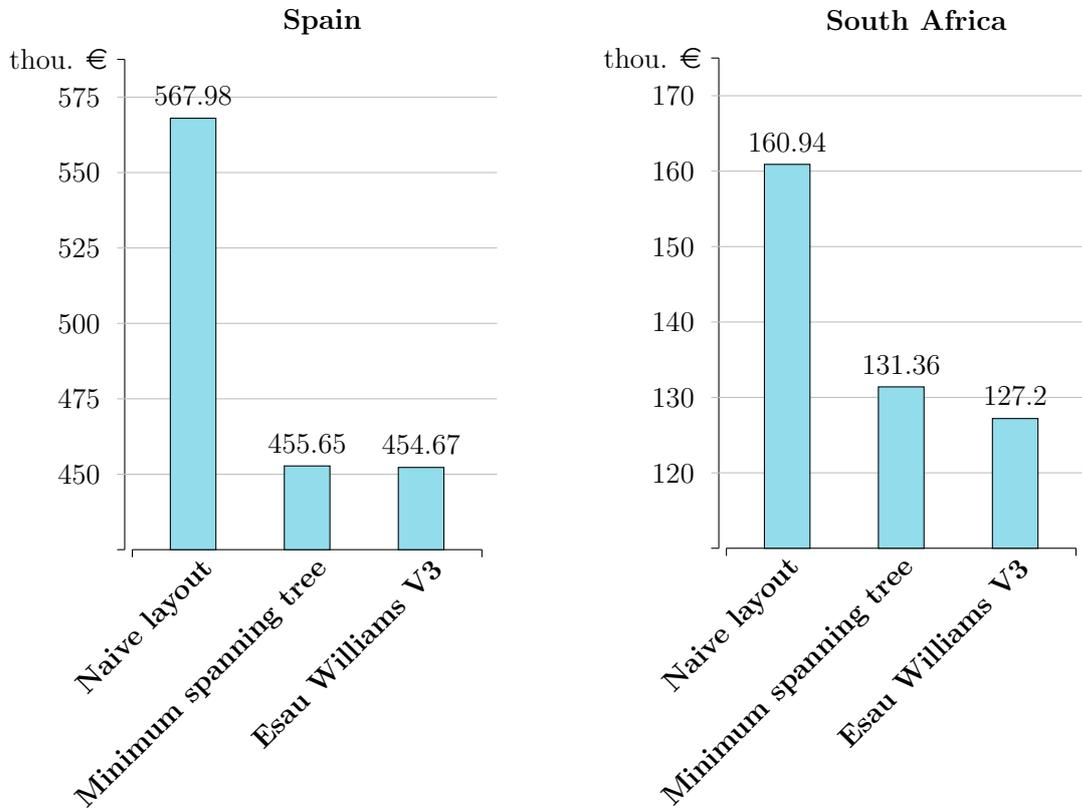
Figure 35: Solar tower: PS10. Comparison of the total costs (in thousand euros) for the power cable dependent on the country the power plant is built in. Note the different axis scaling.
