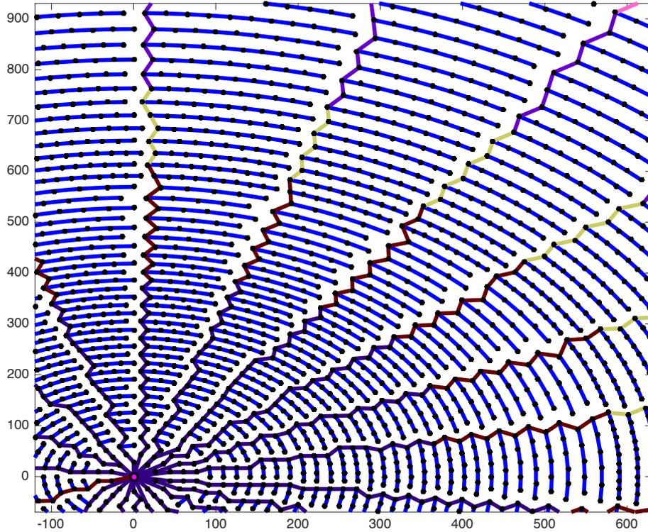
Figure 39: Solar tower: DLR Field, country: Spain. A segment of the naive layout of the power cable for the DLR Field. Different colors mark different cable types.
