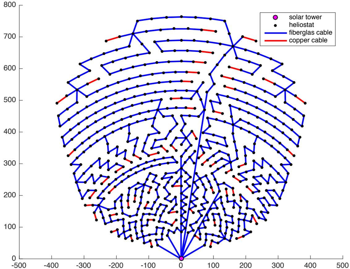
Figure 15: Solar tower: PS10, country: Spain, total cable length: 18 406.24m, total costs: 623 898.38€. Result of Esau Williams Version 1. Blue connections represent cables made of fiberglass, red cables are the ones made of copper.
