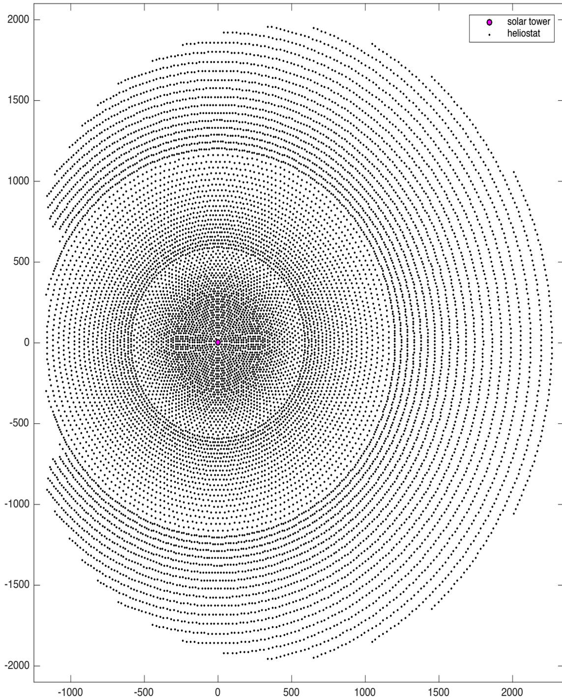
Figure 3: Solar tower: DLR Field. This huge solar tower power plant consists of 12 676 heliostats and a centrally placed tower.
