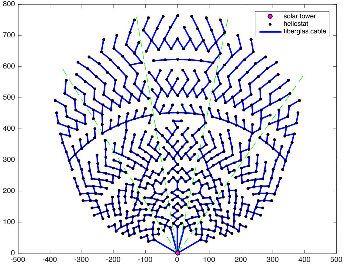
Figure 12: Solar tower: PS10, country: Spain, fiberglass cable length: 16 392.27m, total costs: 596 575.82€. Five minimum spanning trees that connect the heliostats in PS10.
