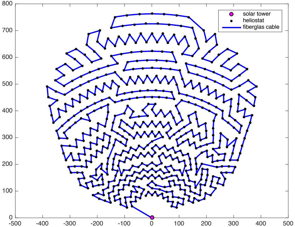
Figure 8: Solar tower: PS10, country: Spain, fiberglass cable length: 16 747.28m, total costs: 548 071.23€. Layout after applying the 2-opt heuristic. All crossings are removed.
