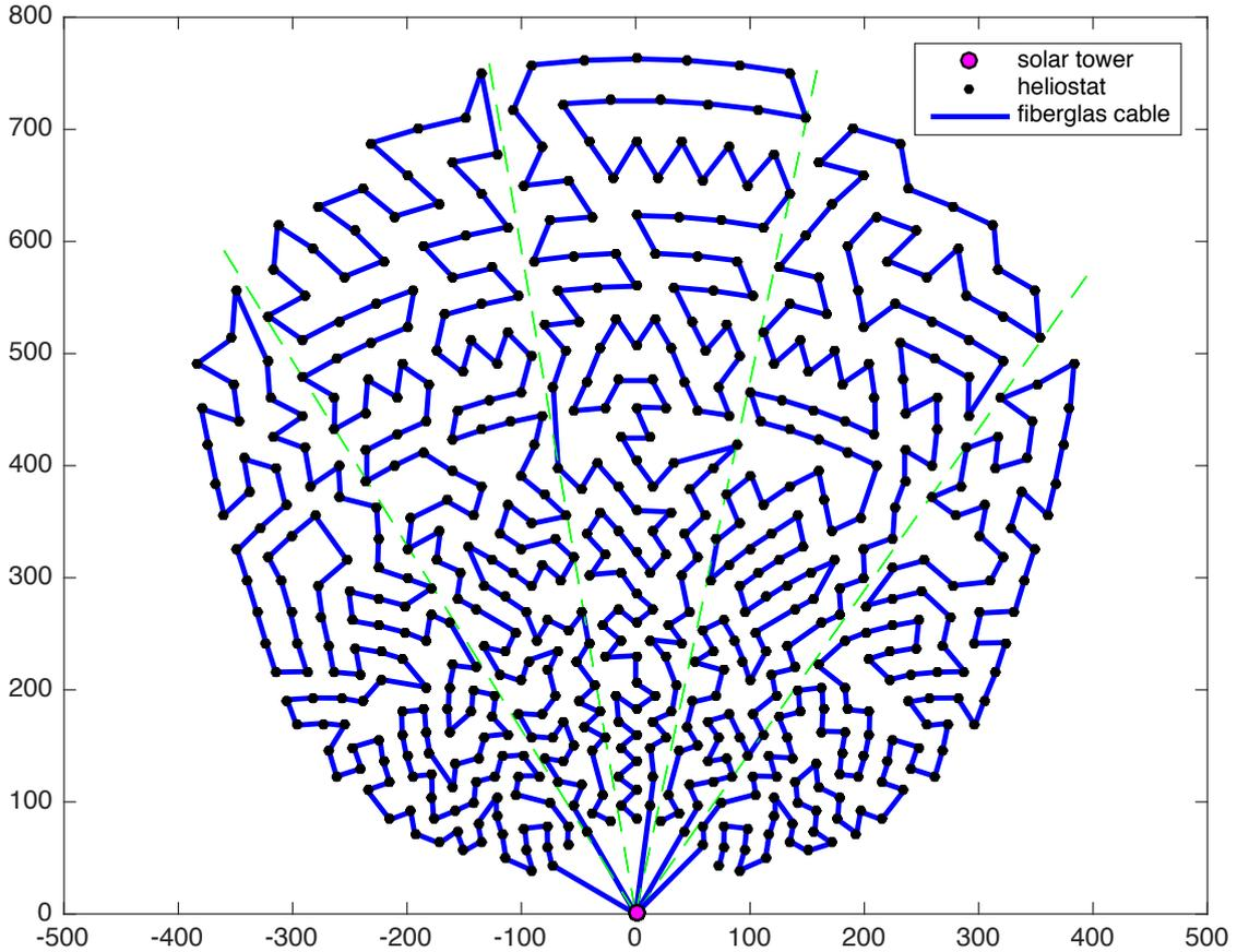
Figure 9: Solar tower: PS10, country: Spain, fiberglass cable length: 17 583.33m, total costs: 572 316.59€. Five Hamiltonian paths made of fiberglass cable starting from the solar tower.
