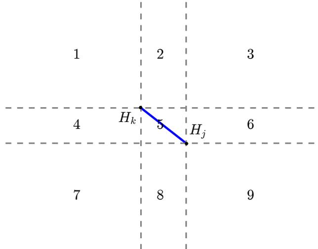
Figure 41: This graphic shows which connections have to be examined in further detail to check for potential crossings. Connections between two heliostats that are placed in the same sector  $m$ ,  $m \in \{1, 2, 3, 4, 6, 7, 8, 9\}$  will not cross with the possible new connection from heliostat  $H_j$  to  $H_k$ .
